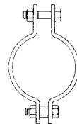
FIG. 216 - PAGE 75 HEAVY DUTY TWO-BOLT PIPE CLAMP WW-H-171-E TYPE 4 A-A-1192 A TYPE 4 MSS SP-58 and SP-69 TYPE 4
