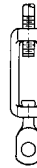
FIG. 114 - Page 56 TURNBUCKLE ADJUSTER WW-H-171-E TYPE 15 A-A-1192 A TYPE 15 MSS SP-58 and SP-69 TYPE 15
