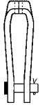
FIG. 909, 909I - Page 110 FORGED STEEL CLEVIS WW-H-171-E TYPE 14 A-A-1192 A TYPE 14 MSS SP-58 and SP-69 TYPE 14
