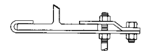
FIG. 156 - Page 64 STEEL BEAM CLAMP WW-H-171-E TYPE 53 A-A-1192 A TYPE 25 MSS SP-58 and SP-69 TYPE 25
