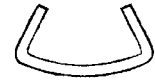
FIG. 1900-1905 - Page 112-114 PIPE COVERING PROTECTION SADDLE WW-H-171-E TYPE 40A & 40B A-A-1192 A TYPE 39A & 39B MSS SP-58 and SP-69 TYPE 39A & 39B
