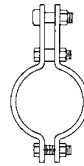
FIG. 189 - PAGE 71 DOUBLE BOLT PIPE CLAMP WW-H-171-E TYPE 3 A-A-1192 A TYPE 3 MSS SP-58 and SP-69 TYPE 3
